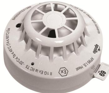
The XP95 I.S. Heat Detector operates by measuring heat levels with a single thermistor which gives a count output proportional to the external air temperature.
